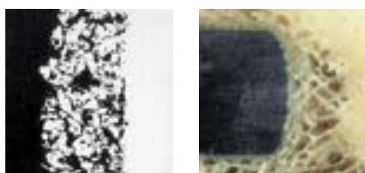
Plasmapore® cross-section and bone contact
